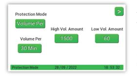
In this mode the system will allow a set amount (volume) of water through the pulse meter during a defined period. By combining these values, you increase/decrease the sensitivity of the systems measurement of flow volume. To edit the flow volume, press the button under the high or low volume value you wish to adjust. Use the arrows to adjust values, press enter to save and return to the screen shown.
