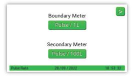
Pulse rates for the water meters connected to the system are selected here. Options available are pulse every: 1, 10, 100 litres.
