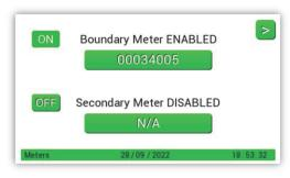
The example shows meter 1 enabled (on) and meter 2 off. If two pulse meters are being used both should be enabled here. To enable, or disable, a meter, press the on/off button on the screen. **The meter values entered should be based on the meter display (converted into litres)**
