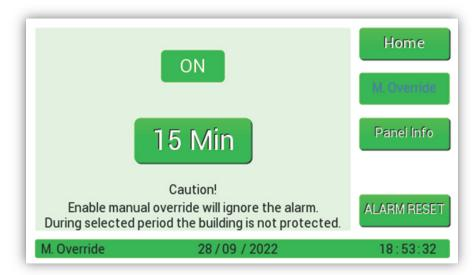
Pressing the ON/OFF button enables the override. There are four pre-set override time periods available. 15, 30, 45 and 60 minutes. Once a time period is selected the "M.Override" button will change to blue and a countdown begins and runs for the selected time period.
