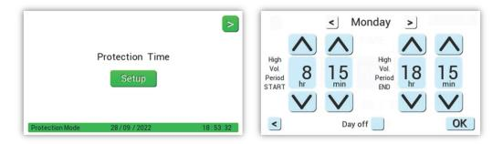
Set the start and end times required for high volume level. Any time outside of the time parameters here are considered low volume levels by the panel and will be measured as such, according to the volume levels selected in Protection Mode: Volume per. Tick 'Day Off' box to ignore that day.
