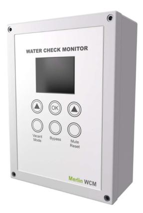
The WCM protects against accidental water leaks caused by burst or leaking pipes. Water flow is continuously monitored and resets every time the flow stops, the user sets the maximum time water flows through the pipes before the supply is automatically shut off. The Vacant mode has alternative settings for early detection, and three zones can be configured with rope or puck leak detection for a complete detection solution.
