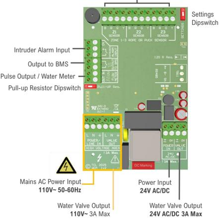
Note: Valve voltage and input voltage must match
