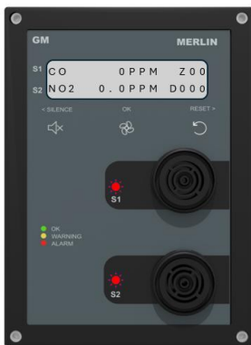
Low Gas Alarm In low alarm the red LED will blink
